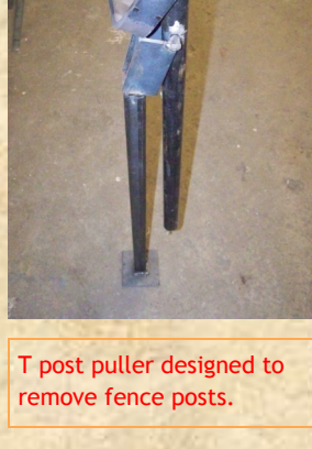
T post puller designed to remove fence posts.
